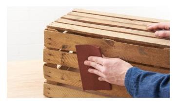
**2.** First clean the wooden box and remove any unevenness with the sandpaper.
